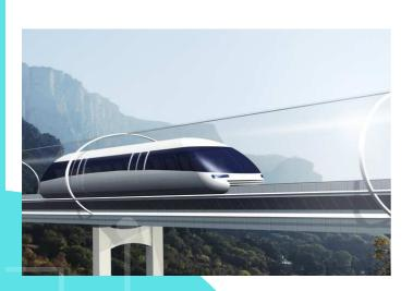
HYPERLOOP IS NEW MODE OF THAT TRANSPORTATION. FREIGHT AND PEOPLE QUICKLY, SAFELY, ON-DEMAND AND DIRECT FROM ORIGIN DESTINATION. **PASSENGERS** OR CARGO ARE LOADED INTO THE HYPERLOOP VEHICLE AND IS ACCELERATED GRADUALLY VIA **ELECTRIC PROPULSION THROUGH A LOW-**PRESSURE TUBE.
